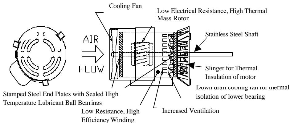
*A high-efficiency ball bearing motor designed for a maximum operating temperature of 450°C helps maintain the very low  $\Delta T$  required for lead-free reflow.*
