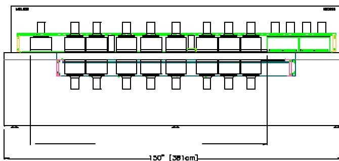
*A nine-zone configuration within the reflow oven ensures the tight gas flow circulation management needed to maintain a consistent lead-free profile.*
