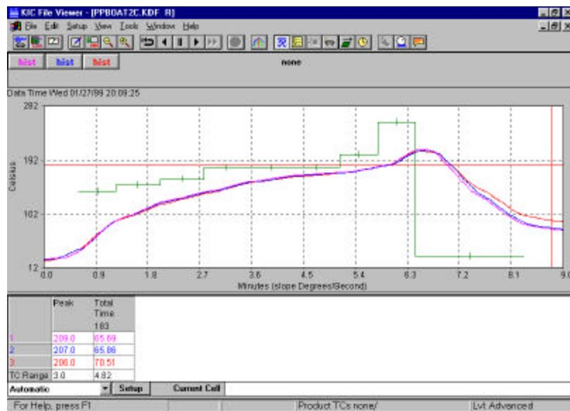
*A typical reflow profile for eutectic tin-lead solder*
